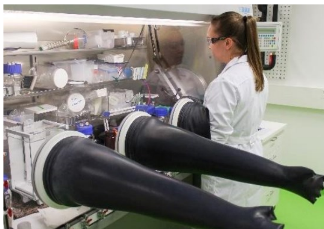
Working with dissolution experiments in controlled atmosphere using a glove box, at VTT
