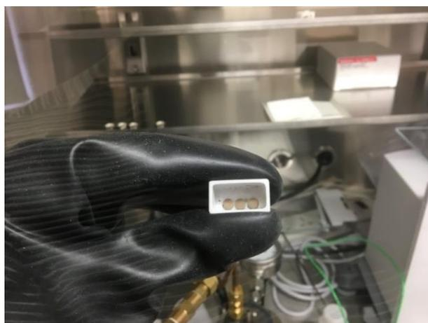
**Figure 2:** Photograph of three sintered pellets of U-Th mixed oxide handled in an anoxic glove box.
