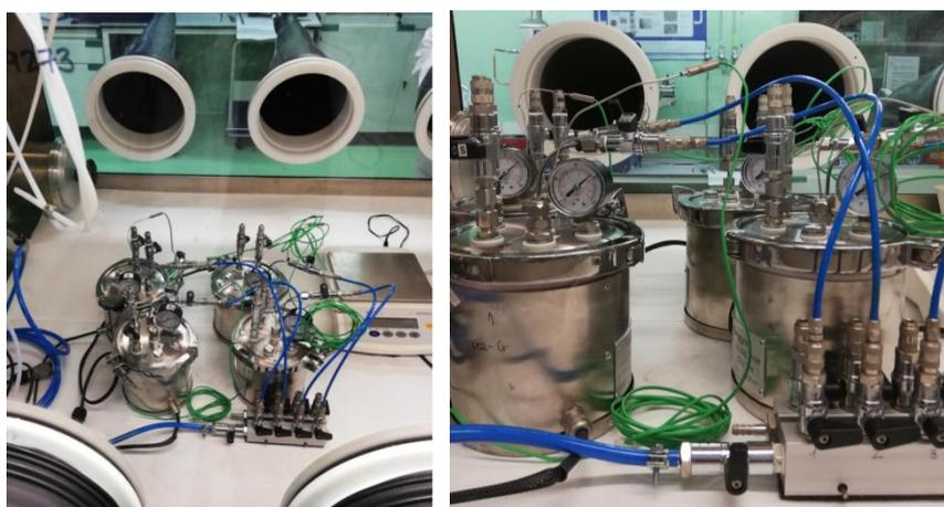
**Figure 3:** View of leaching experimental set up installed at CIEMAT in Ar glove box under 8 bar of 4.7%  $\text{H}_2$ - $\text{N}_2$ .
