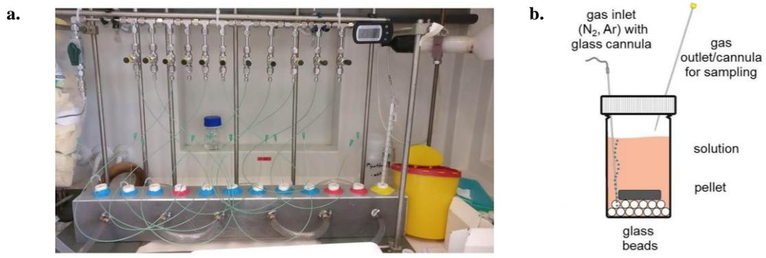
**Figure 4:** (a) Experimental setup of the dissolution experiments. (b) Schematic drawing of the experimental vessels for the accelerated dissolution experiments.
