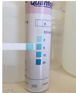
**Figure 4:** Photograph of the semi-quantitative test strips kit used to monitor  $\text{H}_2\text{O}_2$  concentration (for illustrative purpose only).
