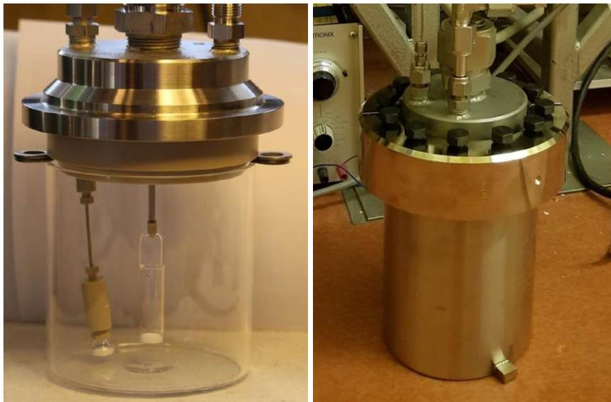
Prior to assembling the autoclaves the free internal volume was determined for gas phase calculations obtaining a value of  $950\text{ cm}^3$ . Leak tests were also performed by pressurizing the autoclaves with 50 bar of He and monitoring the pressure through 1 month. The pressure drop rate found was  $\sim 0.16\text{ bar/month}$ .
