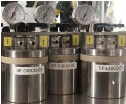
**Figure 2.1.1.1:** Stainless steel autoclaves
