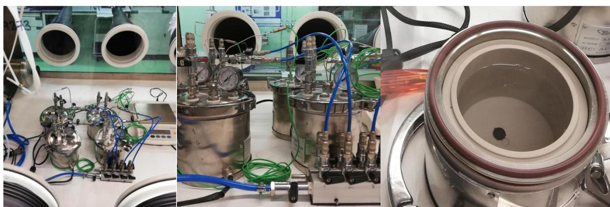
Figure 2.1.4.1.- View of leaching experimental set up installed at CIEMAT in Ar glove box under 8 bar of 4.7% H<sub>2</sub>-N<sub>2</sub>.
