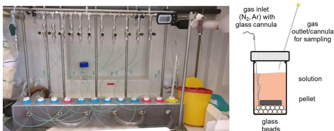
**Figure 2.1.2.1:** (a) Experimental setup of the dissolution experiments. (b) Schematic drawing of the experimental vessels for the accelerated dissolution experiments.
